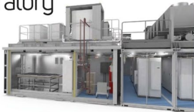
RIGHT: A climatic battery pack test chamber featuring instrumentation space
