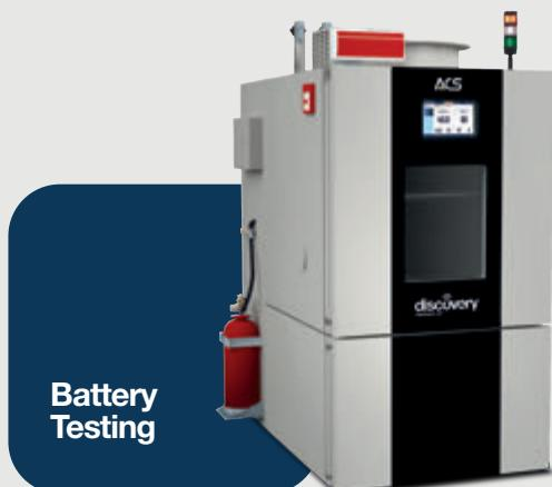
A set of dedicated options is now available for this specific market. Gas detection, protection system and overpressure valves: all devices have been optimized in accordance with the EUCAR Hazard Levels so as to create a standard for safety analyses.
