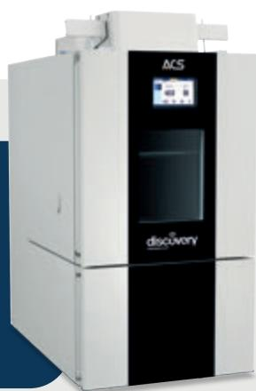
A special lamp array located on the top of the chamber makes it possible to meet the main solar simulation standards, such as DIN 75220, IEC 60068-2-5, ISO 9022-9, VDA 230-219.
